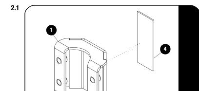
Clean the rear of the Back Bracket (Item1) with Denatured alcohol and adhere the VHB tape (Item 4) to the back of the Mounting bracket.
