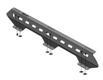
4. Fit 10mm Bolt / Split washer/ Flat washer with the Channel Nuts on top of the rail.
