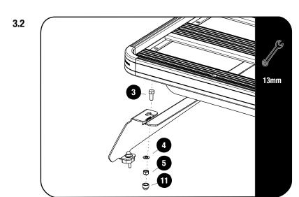
Secure your roof rack to the Foot Rails using M8 x 20 Hex Bolts, M8 x 16 x 1.6SS Flat Washers and M8 Nyloc Nuts (Items 3, 4 & 5).
