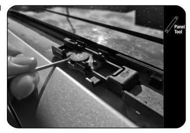
Using a suitable panel tool, remove the ditch moulding on the left and right side of the vehicle.
