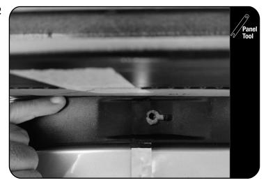
Using a Suitable panel tool, remove the plastic clips at the rear.
