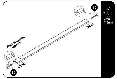
Measure and mark the hole positions on the ditch moulding as shown in 2.3. The positions must be centered on the moulding.
