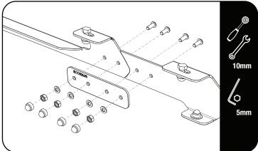
Place the two halves of the foot rail on to the spacers and join the 2 halfs with the supplied splice plate Item 8. Fasten as shown with Items 9, 10, 11.
