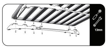
Fit and secure your roof rack to the foot rails with items 14, 15 and 16.
