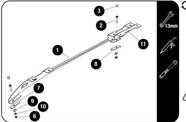
Apply a bead of sealant on the threads of the M8 x 40 Hex Bolts and secure the Foot Rail (Item 1) together with the Support Bracket (Item 11) and the Front and Rear Spacers to the Roof using M8 x 40 Hex Head Bolts, M8 x 19 x 2 Flat Washers and M8 Nyloc Nuts (Items 2, 6 & 10).
