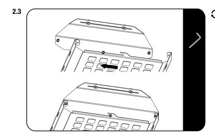
with the Front Runner sticker facing the rear of the vehicle, align the mounting slots on the Internal Cargo Tray (Item 1) with the M6x12 Button Head Bolts and slide the tray into position as seen in Fig 2.3.
