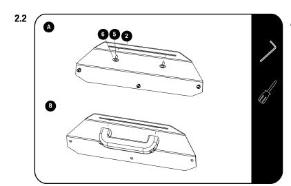
Remove the rear grab handles in the vehicle by removing two mounting screws. Fit the side brackets (Item 2) using the grab handle mounting points. The side brackets can either be fitted using the M6x16 Button Head Bolts (Item 5) and the M6 x19 x 1 Flat Washers (Item 6) as seen in Fig 2.2A, or it can be mounted by refitting the grab handle as seen in Fig 2.2B.
