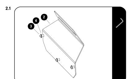
Insert the M6 x 12 button head bolts (Item 3) and M6 x 12 x 1 Flat washers (Item 4) into the side brackets (Item 2) as shown but do not thread all the way.
