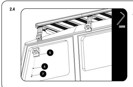
Secure the Gutter Clamps (Item 5) using M8 x 30 Button Heads and M8 Schnorr Washers (Items 6 & 7).
