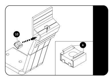
Secure the M8 Cage Nut (Item 10) to the inside of the aluminium leg's cavity with the flanges (A) facing outward.
