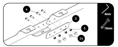
Join the two halves of the Foot Rails (Item 1 & 2) with the supplied Joiner plate (Item 3). Use the M6 x 16 Button Head bolt, M6 Nyloc Nut and M6 Nut Cap (Item 4, 5 & 14) and Fasten as shown.
