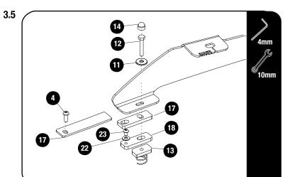
Apply a bead of silicone on each Hex Bolt inserting it into the roof.
