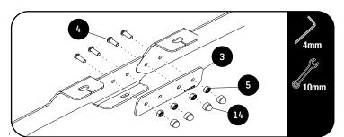
Join the two halves of the Foot Rails (Item 1 &3) with the supplied Joiner plate (Item 3). Use the M6 x 16 Button Head bolt, M6 Nyloc Nut and M6 Nut Cap (Item 4, 5 & 14) and Fasten as shown.
